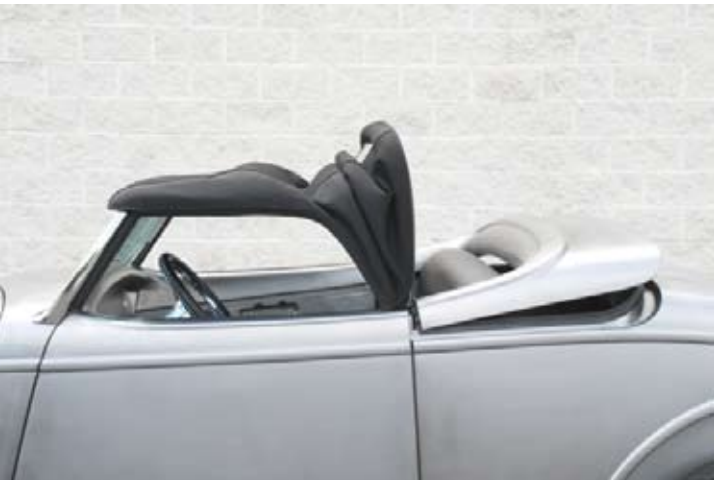
The now-you-see it, now-you-don't top is the best part of ASC's Speed33. Stowage begins by lifting the rear of the top and opening the tonneau cover/tulip panel. First, the rear of the panel rises ...
