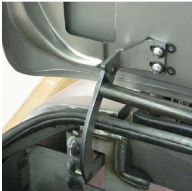
The tonneau cover also goes through a variety of moves when opening. This is the hinge assembly at the back of the panel.
