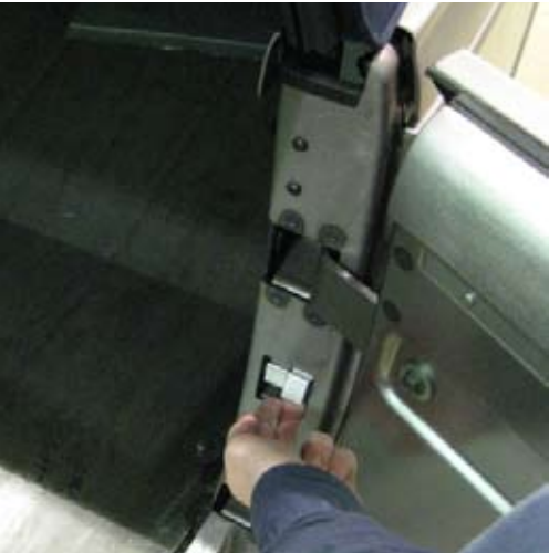
Release latches for the tonneau cover and the trunk lid are in the hinge post. Note the hidden hinges.
