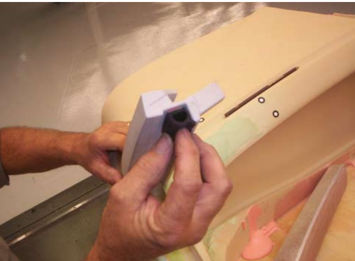
One of the greatest challenges had to be the windshield posts, which had to be slim and stylish while incorporating channels for roll-up windows. Production versions are investment-cast in stainless steel.
