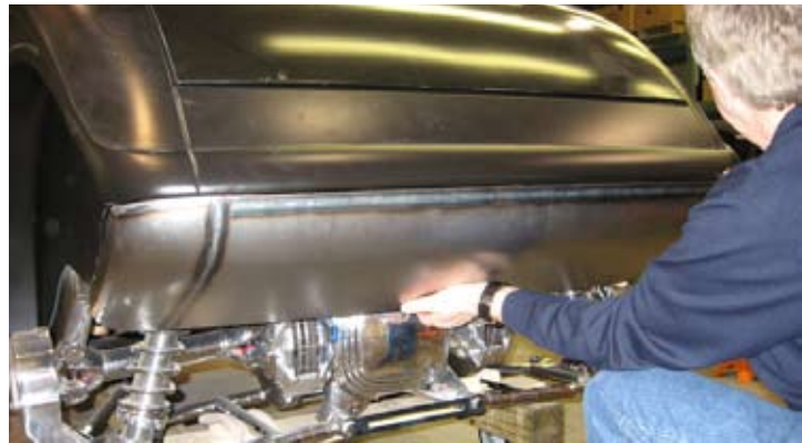
Speaking of options, a rolled rear pan will be used on the '08 Road Tour car. The fuel tank will be in the trunk.
