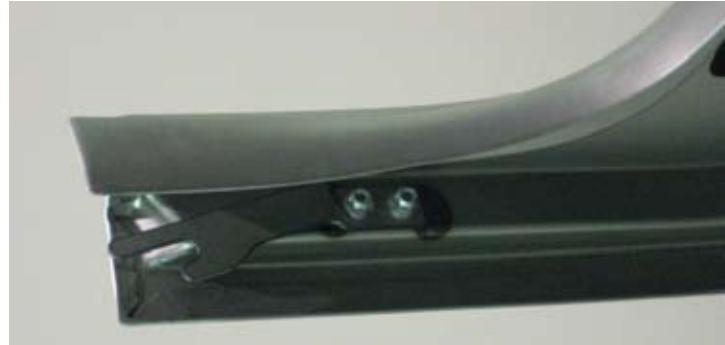
This is the right side catch that secures the front of the tonneau cover when it's in the closed position.
