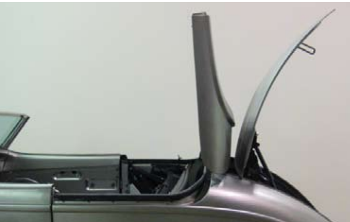
This took some engineering: The tulip panel/tonneau cover can be opened at the same time as the trunk lid. The leading edge of the trunk lid moves to the rear as it opens.
