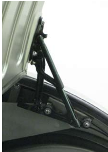
This is the right side catch that secures the front of the tonneau cover when it's in the closed position.
