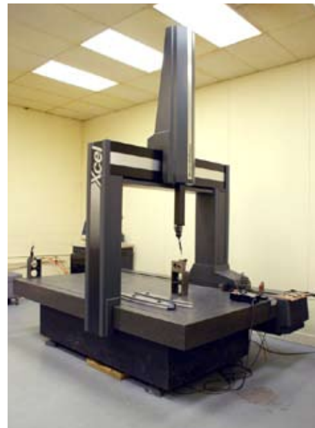
This digitizer is used to pick up datum points and prove the dimensional accuracy of the computer model. If changes are necessary, they can be made before production begins.
