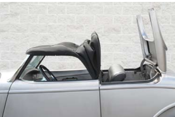
... then it moves to the rear, the front disengages from its guides, and the panel opens fully.
