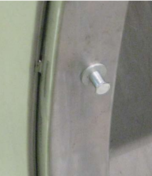
As you would expect, the Speed33 is equipped with modern, bear-claw door latches. This is the pin in the latch post.
