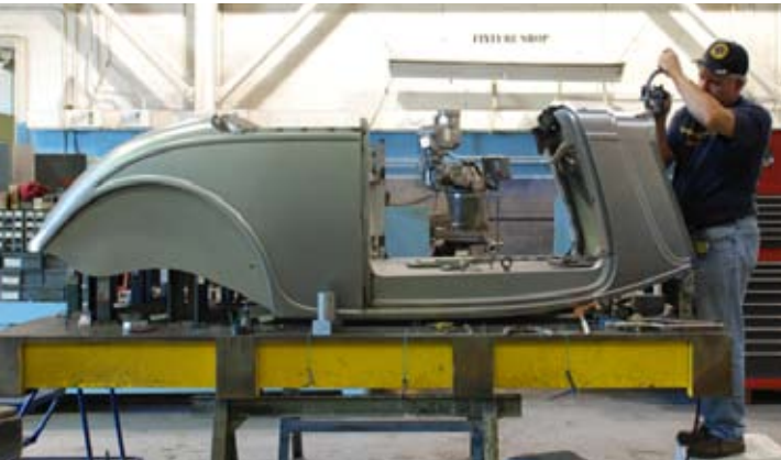
Bodies are assembled on a surface plate to ensure proper panel alignment, and gaps are established to OEM tolerances. E-coat (electrocoating cathodic epoxy) dipping is also available to protect your investment.
