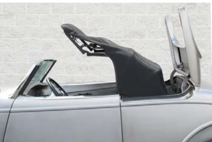
With the windshield latches released, the header assembly can be moved up and back.
