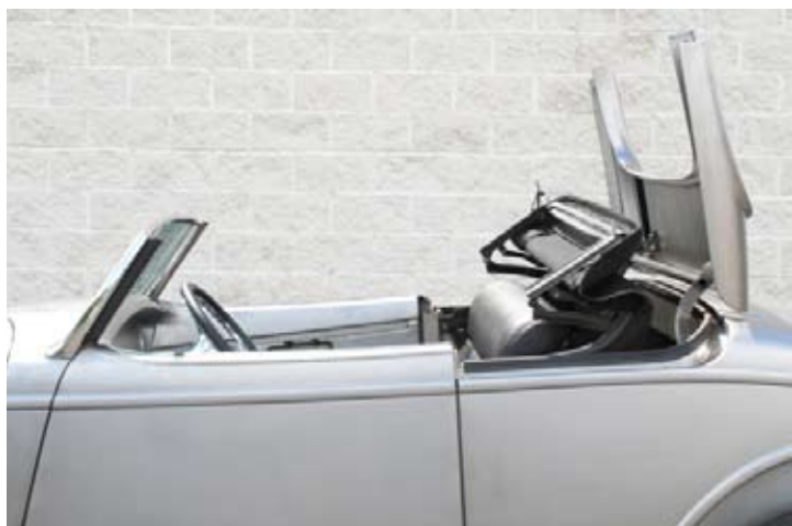
The top assembly folds easily and is completely hidden in a well behind the seats.
