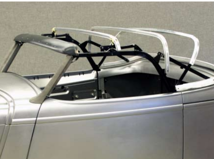
Here's a good look at the top bows before the Haartz cloth material was put in place. Tops are available in black, beige, and navy blue, as well as custom colors.
