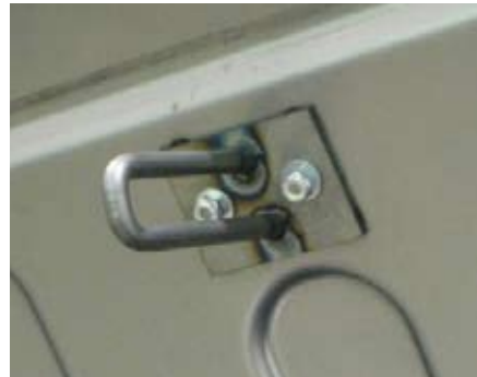
More modern hardware can be found securing the trunk lid in the closed position.
